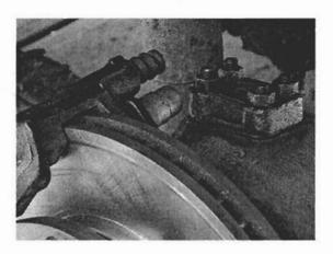
. The oil level in swivel ball housing should be checked and the oil replaced or topped up as necessary. Remove protective coating from disc (rotor) surface with brake cleaner.
