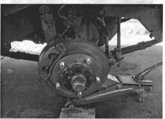
Bleed brakes as per the Land Rover Service Manual Tighten bleed valve to 62 inch/lbs.
