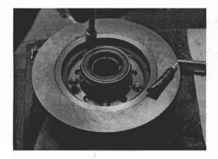
Mount disc (rotor) to hub using the five (5) metric 10mm x 1.5 fasteners provided. Apply one drop of Removable Thread Locking Compound to each fastener before installation. Tighten fasteners to 50 ft/lbs.
