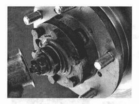
Attach driving flange, (or free wheeling drive systems if fitted) to hub using retained fasteners and reinstall drive axle retaining nut. Use new gasket and seal provided and tighten to Land Rover specifications.
