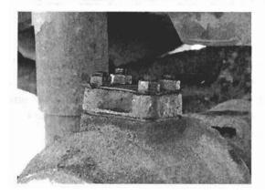
Clean the area around the upper swivel pin and remove (4) four upper swivel pin bolts (or studs if so equipped).
