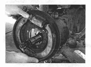
Carefully remove brake backing plate complete with brake shoes, cylinders and brake hose.
