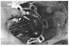
Remove wheel hub retaining nuts and locking ring.
