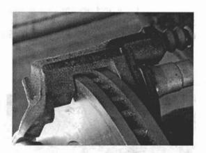
Remove swivel housing oil filler plug. If, during removal, the filler plug interferes with the caliper mounting bracket fastener, it should be shortened. The amount to be removed (if any) will vary for each filler plug (typically 3/16" is required).
